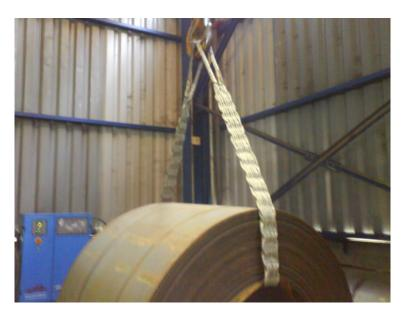
They are slings from wire ropes for heavy load and fragile cargos. For example coil steel, hot rolled, big rocks, marbles, vessel e.t.c
